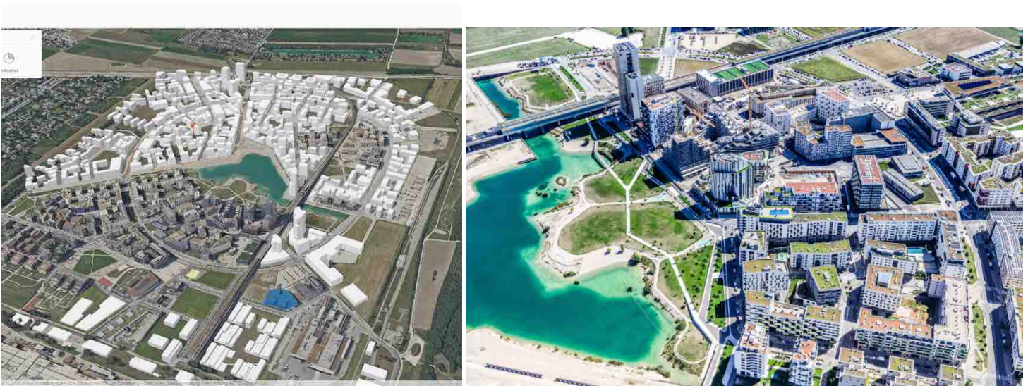
Aspern Seestadt on a brownfield site on the outskirts of Vienna, Austria. Transit oriented suburban development with Phase I completed. A walkable bikable neighborhood serviced by a train station with a 40-40-20 circulation split (40 public transportation, 40 walking and 20 personal vehicles). Final buildout by 2030 targets housing for 25,000 people and 20,000 jobs all within 800 acres. Source: ESRI blog
