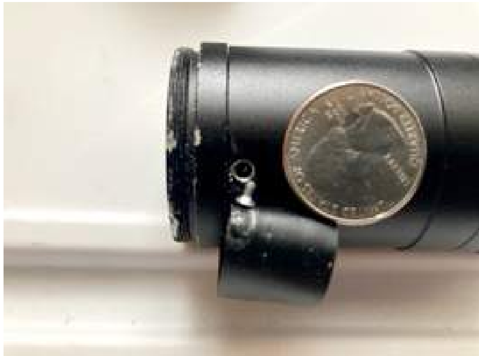
Case #5 One tiny screw shear and the magnification feature is lost.
