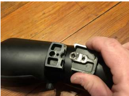
Case #1 Broken mount (top) and fracture across threaded hole (bottom).
