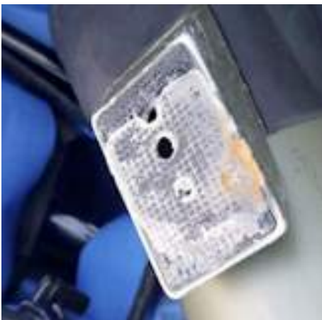
Case #2 Stripped and damaged threaded hole in aluminum.
